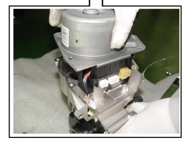
Remove the original flexible coupling (O) from the housing. In addition, use an air gun to remove any foreign matter from the motor and/or the housing.
