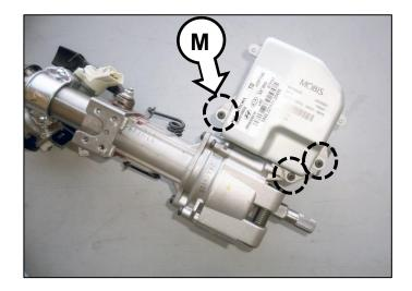
10. Remove the 4 Torx<sup>®</sup> head screws (N) securing the MDPS motor cover.
