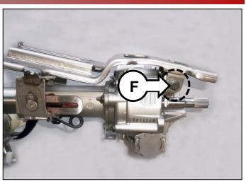
5. Remove the steering column guide bracket (G) from the steering column.
