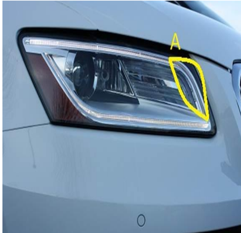
Figure 5. Upper light pipe perceived defect (A).
