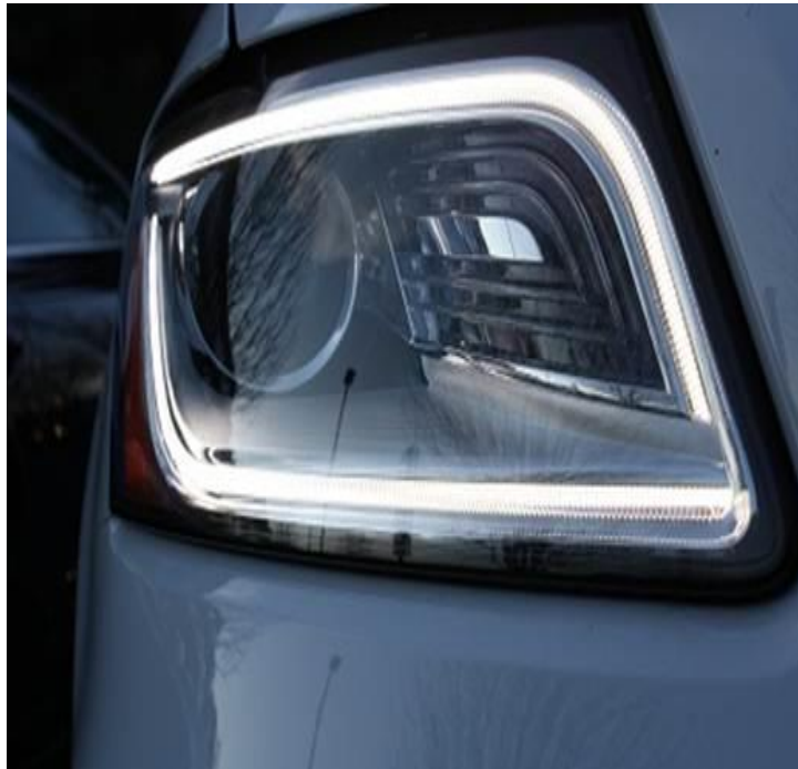
Figure 1. Upper and lower light pipes illuminated.
