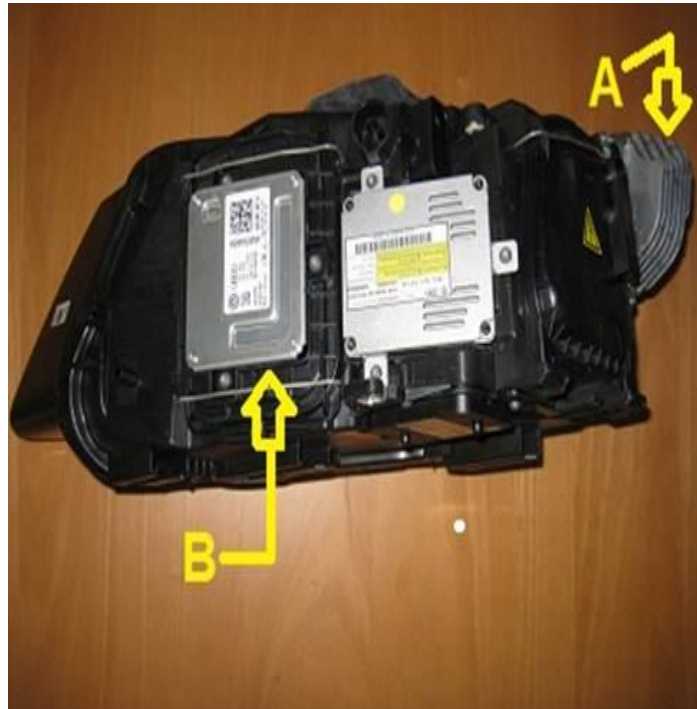
Figure 2. The backside of the headlight with LED heat sink (A) and LED control module (B).
