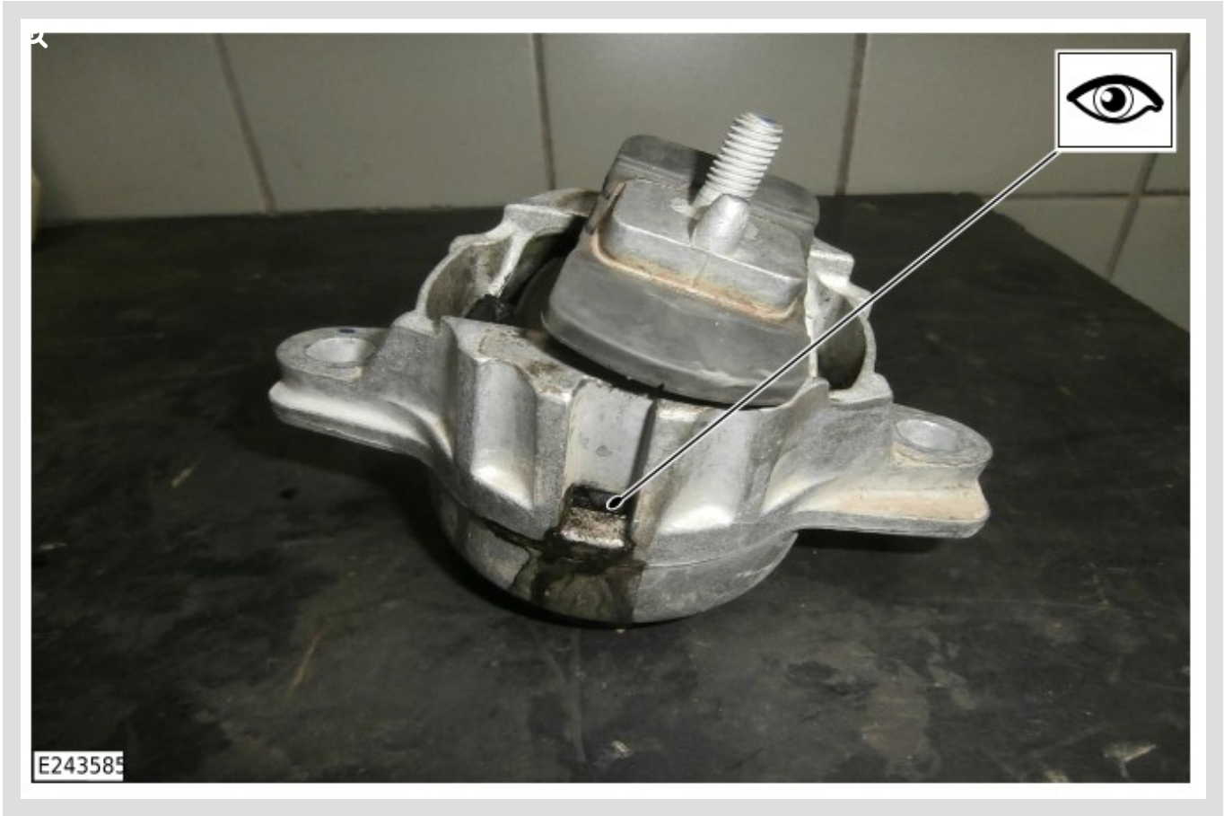
Excessively worn and/or leaking active engine mount.
