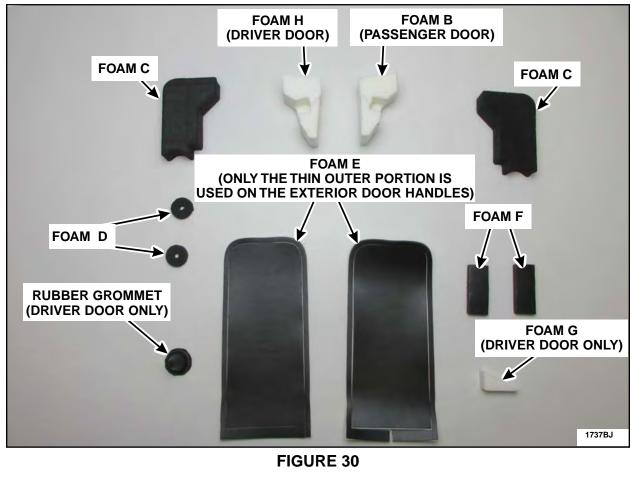
1. For driver door latch only, attach Foam G to Foam H. See Figure 31.
