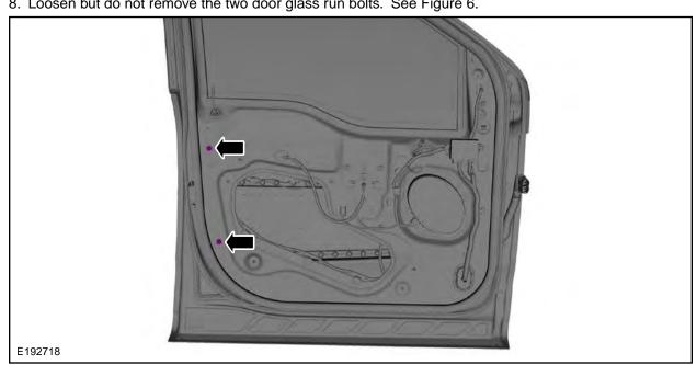
8. Loosen but do not remove the two door glass run bolts. See Figure 6.
