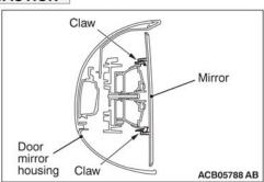
The tab of the mirror is prone to breakage when working in cold temperatures. Always use a hair drier or the like to warm up the mirror tab and its periphery to 20°C or higher prior to works. When the mirror is heated too quickly from its cold state, it may be broken.
