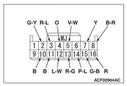
Check the wire colour of the wiring harness, and insert it into the connector as shown in the illustration.
