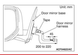
2. Fix the base assembly and the wiring harness at the position of the specified length with a new tape.
