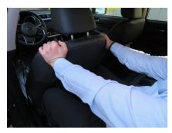
**Step 3-** While sitting in the driver's seat, apply pressure with feet / legs as shown towards the back of the seat while leaning and shifting body weight towards the four TORX bolts. When complete, raise the seat to the fully lifted position.
