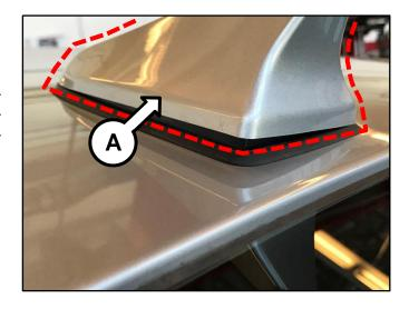
2. Remove any remaining plastic remnants from the screws at the antenna base (B) and then using regulated shop air, gently blow and clean the rubber padding of the base.
