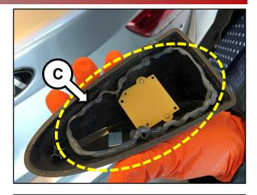
5. Carefully align and place the antenna cap over the antenna base. Firmly hold the cap onto the base for fifteen (15) seconds.
