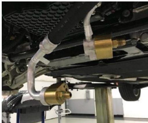
Figure 6. Installation of VAS 6338/3 and 6338/12.
