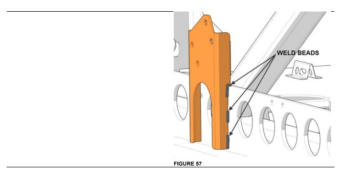
48. As a preparation to **welding**, use a grinder with abrasive disc to remove some paint to reach bare metal. Weld the **ground stud** #380360 centered in the beam and at 14 inches from the beam end.
