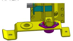
FIGURE 21: MOUNTING SUPPORT AFTER 180° ROTATION
