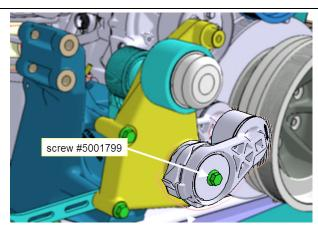
FIGURE 46: TENSIONER MOUNTING SCREW TORQUE : 48 lb-ft
