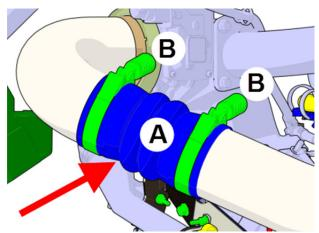
Constant Torque hose clamps 4.25in - charge air cooler (CAC) 4.5-5.5 lbf-ft
