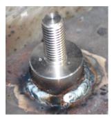
49. Apply black paint to the area surrounding the ground stud and the ground stud circular base. **DO NOT** apply paint on the electrical contact surfaces.
