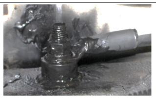
FIGURE 80: GROUND STUD WITH RUBBER COATING
