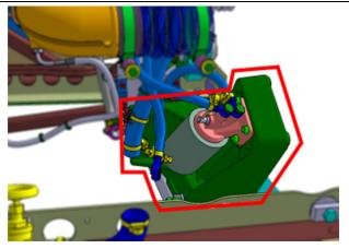
FIGURE 31: L.H. REAR ENGINE SUPPORT
