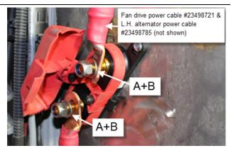
FIGURE 153: TAKE NOTE THAT THE 300A FUSE IS NOT SEEN ON THE PICTURE ABOVE BUT IT SHOULD BE INSTALLED AT THIS STEP
