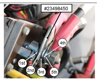
FIGURE 151: ON THIS PICTURE, CABLE #23498450 LUG IS IN SECOND ( $2^{\rm ND}$ ) POSITION BECAUSE IT WAS LIKELY TO RUB ON THE HEAD OF ONE OF THE FOUR SCREWS.
