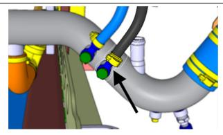
FIGURE 71: DEF INJECTOR COOLANT LINE RETURN HOSE
