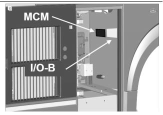
FIGURE 156: MAIN POWER COMPARTMENT
