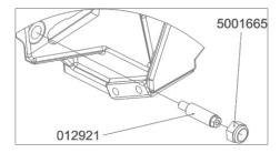
FIGURE 36: REAR VIEW - GROUND STUD
