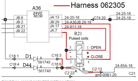
FIGURE 24: 062305 HARNESS INSTALLATION
