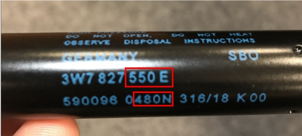
Correct right hand side strut 3W7827550E (480N) - marked in Blue writing.
