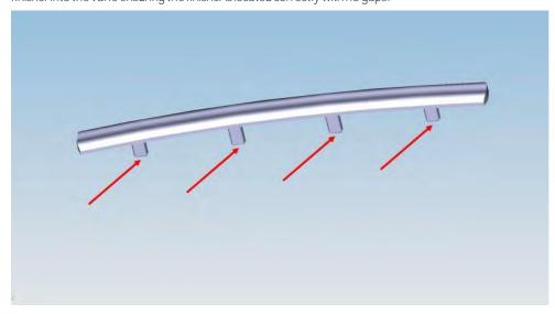
Note: Rotate the vane to the fully down position or fully up position, the vane in this position gives the maximum clearance between the ends of the vane finisher & the bull seye trimring during re-fitment.
