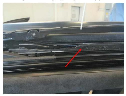
• The above illustration shows the right mechanical system from the inside. Here is the groove (see arrow) which also has to be sprayed once or twice.
