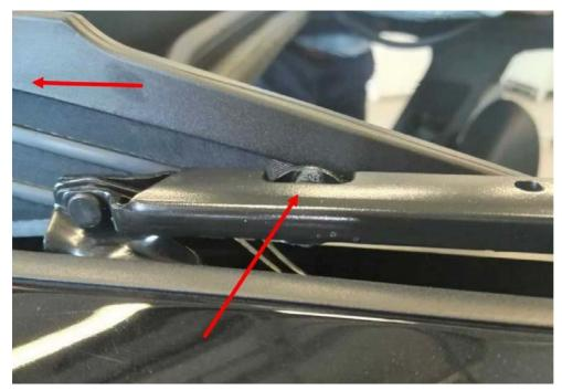
2) The above illustration shows the left mechanical system. The upper left arrow points to the driving direction. The lower arrow points to the first mounting point of the glass panel.
