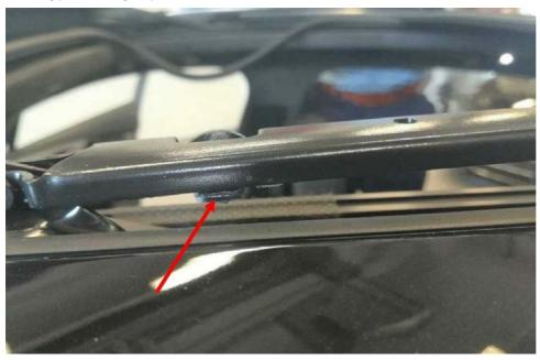
• There is a lug under the first mounting point (see arrow). This should be sprayed once or twice.
