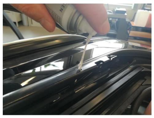
• The above illustration shows the left front mechanical system. Here the point to be lubricated which can be reached with the nozzle via the first hole in the lever.
