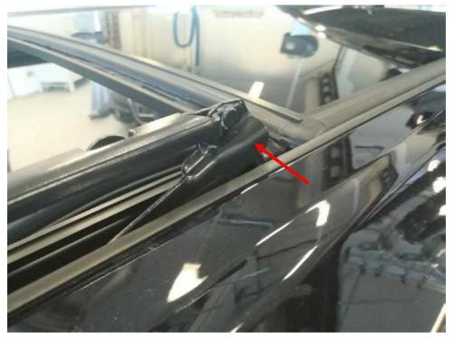
• The above illustration shows the left mechanical system which also has to be lubricated in the outer rear area (see arrow).
