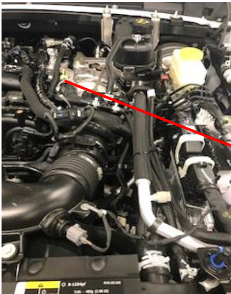
Under-hood View of Upper Radiator Hose Clamp Grenade Pin Still Attached.
