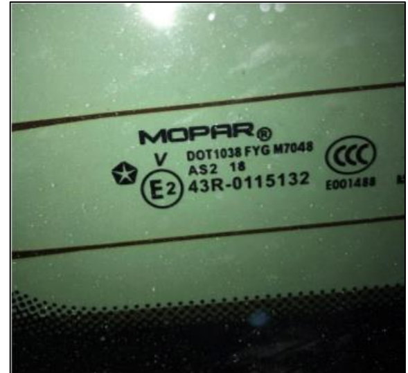
Figure 2 – Example of Acceptable Photograph of Backlite AS2 Marking
