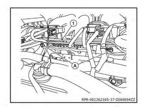
16. Loosen bolts in reverse of sequence shown and remove electric throttle control actuator bolts, then remove electric throttle control actuator and position aside.
