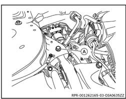
21. Remove fuel tube bolts (A).
