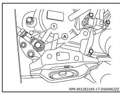
64. Remove water hose (1) from retainer (A).
