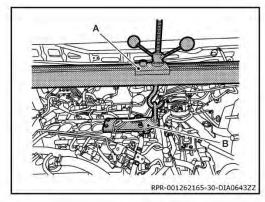
29. Using bubble level (B) on Tool (A) level Tool as shown. Refer to Engine Support Tool Operating Instructions.
