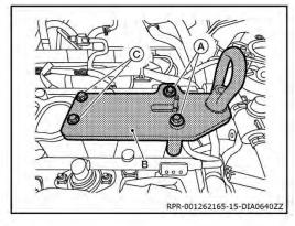
26. Install Tool (A) to drivers side frame rail (1) as shown. Refer to Engine Support Tool Operating Instructions.
