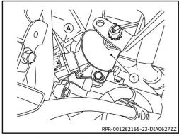
6. Disconnect brake booster vacuum hose from intake manifold collector. Refer to Vacuum Lines "Exploded View" in the Brake System section of the ESM.
