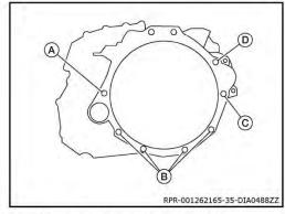
81. Separate the transaxle assembly from the engine assembly and lower transaxle assembly.
