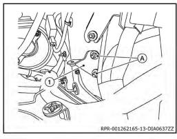
25. Install Tool (B) using bolts (A) and (C) supplied with Tool. Tighten bolts to specification. Refer to Engine Support Tool Operating Instructions.
