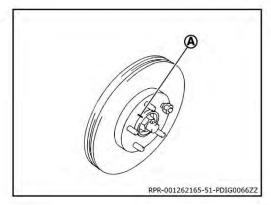
36. Remove wheel sensor bolt (A) and position wheel sensor aside (LH/RH).
