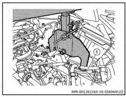
Install Tool (A) on top of engine mounting insulator [RH (1)] as shown. Refer to Engine Support Tool Operating Instructions.
