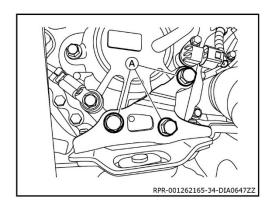
63. Remove bolt (A) and position ground (1) aside.
