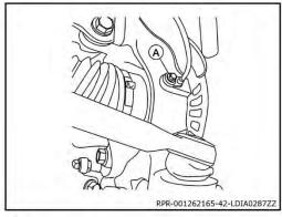
37. Remove and discard cotter pin from front drive shaft (LH/RH).
