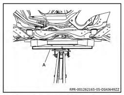
67. Remove front suspension member bolts and front suspension member stays. Refer to Front Suspension Member "Exploded View" in the Front Suspension section of the ESM.
