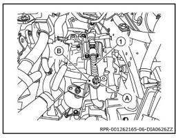
5. Disconnect the harness connector (A) from the transmission range switch (1).
