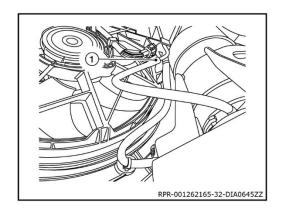
57. Remove bolt (A) and remove rear cover plate (1).
