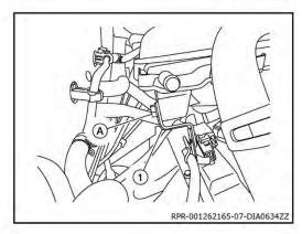
18. Loosen the intake manifold collector bolts and nuts in reverse of the sequence shown, then remove the intake manifold collector and gasket.
