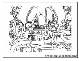
9. Disconnect vacuum hoses (1) from intake manifold collector (2).
