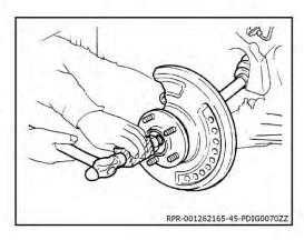
42. Remove the wheel hub lock nut (LH/RH).
