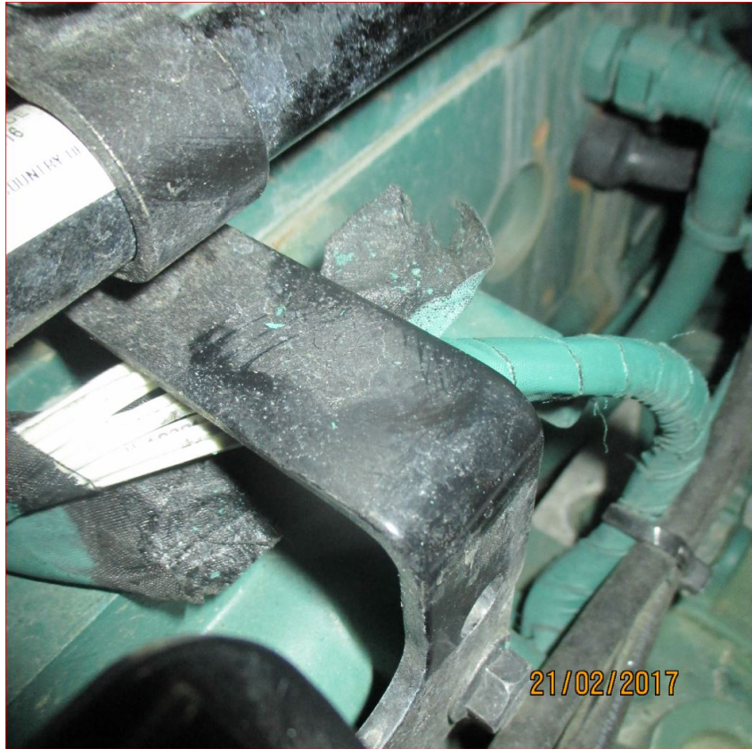
VCB circuit wire with rub fatigue
