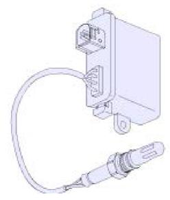
Installation torque of 50 Nm +/- 5
