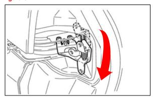
B. Install the center hinge with the three bolts.
