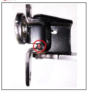
Watch the scribe lines while manually moving the slide door forward and backward until just BEFORE the closed position and when the center hinge pivots.
