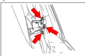
C. Using a brush, apply an anti-rust coating to the center hinge, as shown.
