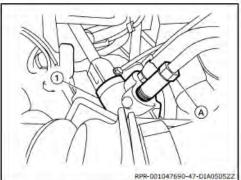
65. Remove lower bolt and separate the steering intermediate shaft from the steering gear.
