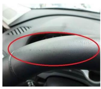
Figure 2. Example of damage from external impact.
