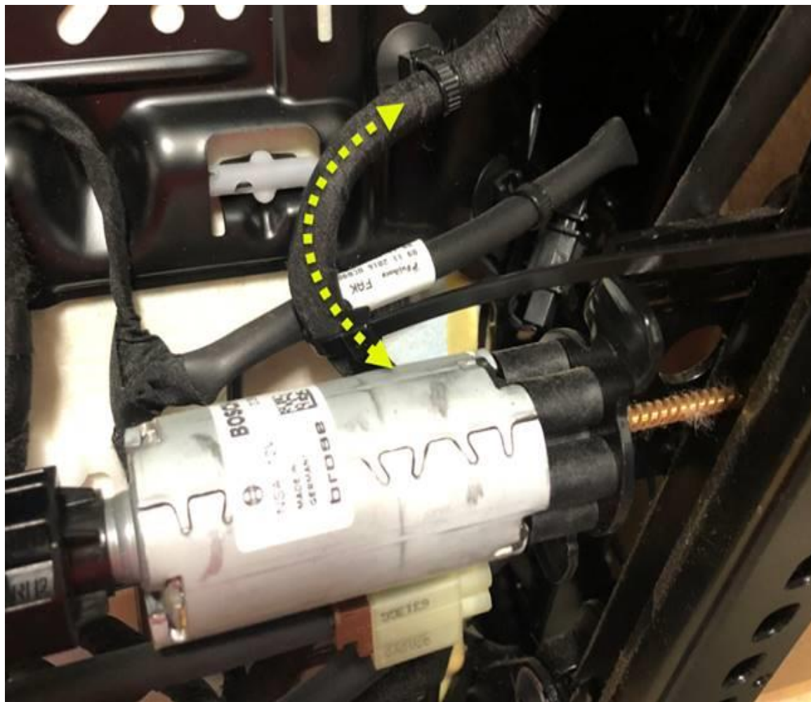
Figure 3. Attach the second cable tie to the yellow marked area.
