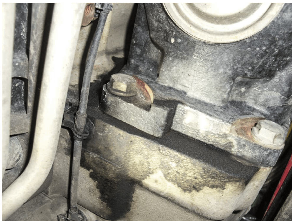
Figure 2. Example of a Seep - Residue Accumulation on the Surface But Remains on that Surface and Does Not Drip onto the Ground
