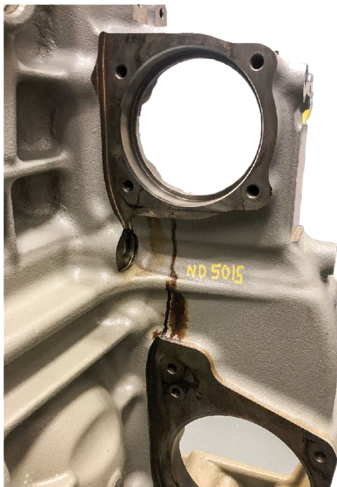
Figure 6. Example of Assembly Grease Residue around High Pressure Fuel Pump
