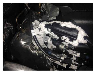
Figure 1. Evidence of leak—AdBlue residue.
