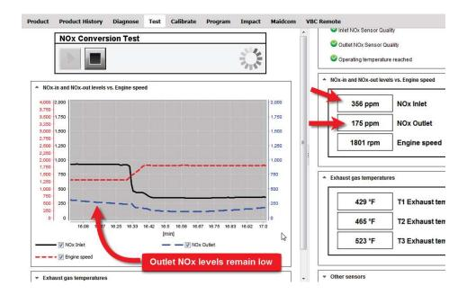
In this instance, review earlier sections of the test to ensure that both sensors are responding to changes in the same manner. Examples of different stages to review are shown below.
