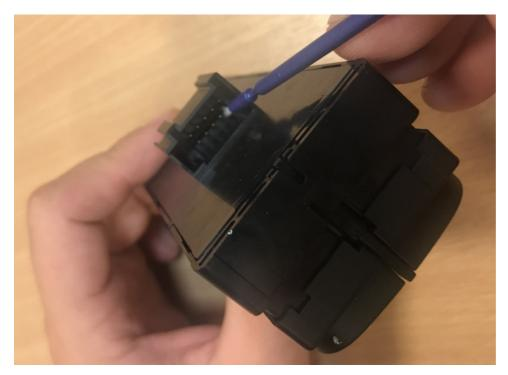
Allow 2-3 minutes for the Isopropanol/ethanol to evaporate (if used) which will leave a thin layer of Stabilant 22 on the connections.
