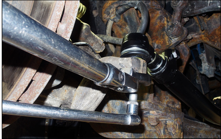
FIGURE 10: BALL JOINT TIGHTENING
