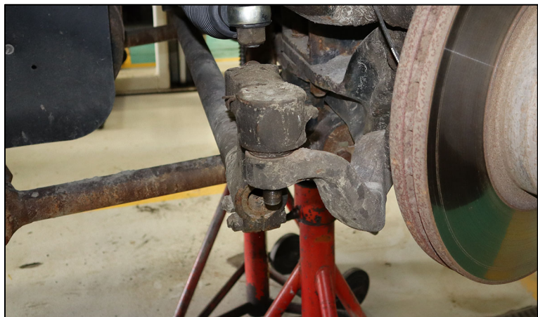
FIGURE 4: BALL JOINT DISSASSEMBLY
