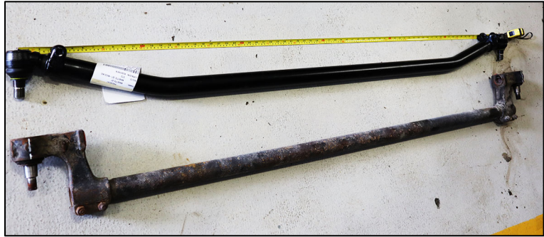
FIGURE 7: NEW TIE ROD LENGTH ADJUSTEMENT
