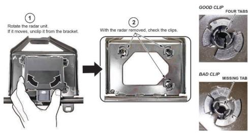
These items should be checked first before replacement of the radar unit. If you are still having issues after following this, then replace the radar unit.
