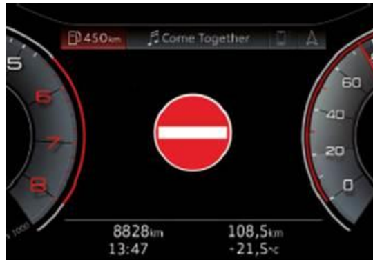
Figure 1. Wrong way traffic sign in the instrument cluster.
