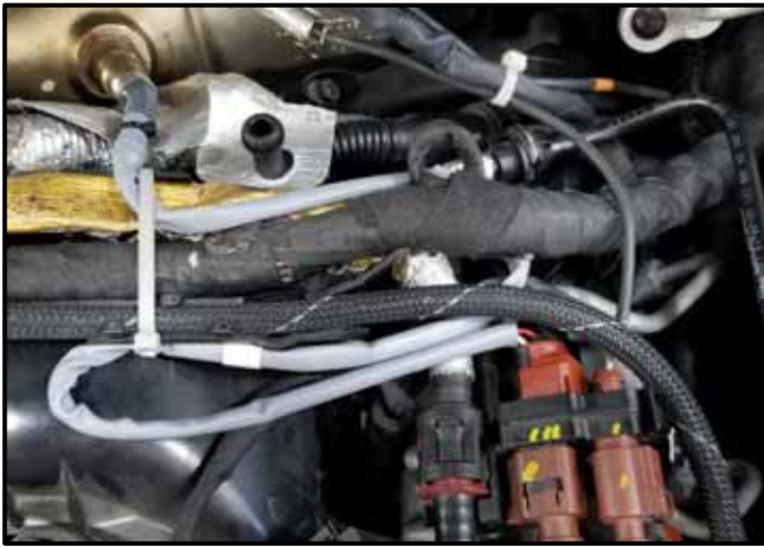
O2 sensor wiring harness routing procedure and tie strap installation
