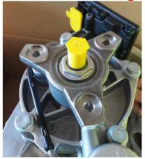
If letters/numbers are present, serial numbers on the backside of the flange are to be checked. Serial numbers greater than 100021A19 (January 21st 2019) are correct.
