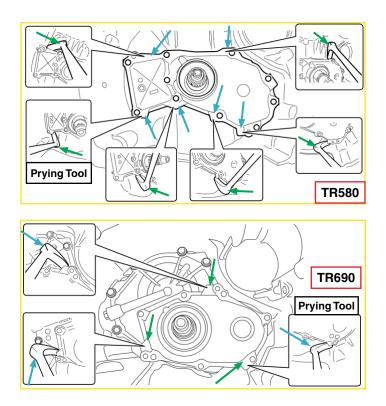
• CAREFULLY remove all residual sealant completely from the cover and mating surface of the housing. DO NOT use any abrasive or gasket removal / cleaning discs. Use the adhesive side of a piece of duct tape (or equivalent) to pick up any loose pieces of sealant material which may be found in the cavity around the stator support. DO NOT use compressed air.
