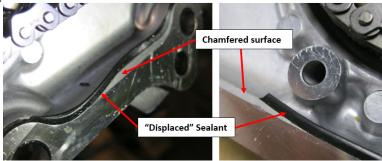
Inspect both of the machined sealing surfaces closely for irregularities. If necessary, replace the cover following the applicable Service Manual procedures.
