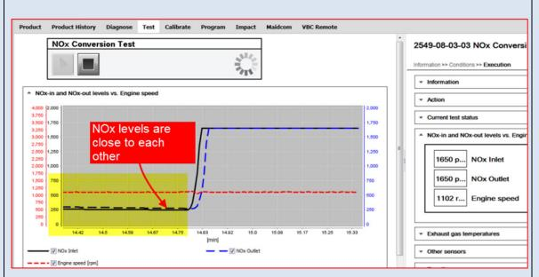
The NOX sensors levels are close to each but earlier during the test (images above & below).
