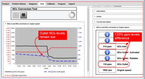
**DIFFERENT BEHAVIOR.** In this example, the NOx sensors ppm levels are not close to each other because DEF is still injected during the last part of the test. **In this instance**, **review earlier sections of the test** to ensure that both sensors are responding to changes in the same manner. Examples of different stages to review are shown below.
