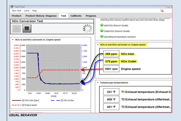
If both NOx sensor ppm levels are **close to each other** during the last part, as shown in the example above (image), then both NOx sensors are good.
