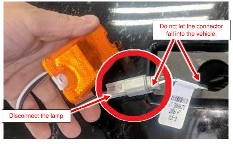
Disconnect the marker light. Do not let the Deutsch connector fall into the vehicle.
