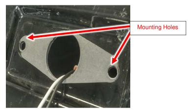
Using warm water and soap, or a suitable adhesive remover, clean the marker light area completely.
