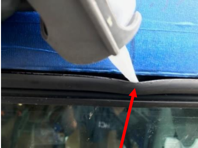
Apply Urethane between fence and front cap.
