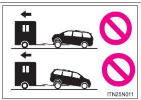
AWD models: Never tow this vehicle with any of the wheels on the ground. This may cause serious damage to the transaxle and Active Torque Control 4WD system.
