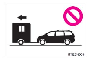
Do not tow your vehicle with four wheels on the ground.
