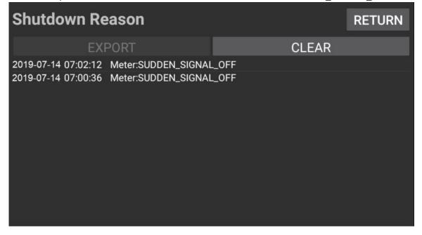
There was a complete loss of signal on the network between the meter (gauge control module) and the previous transmitting unit on the network. In this example, the previous unit is the tuner or tuner-amplifier unit. Although the specific cause is not identified, the failure was confirmed, and the components and connections that should be inspected have been isolated.
