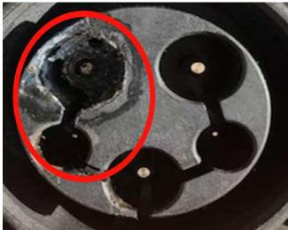
3. Pictures of charge port receptacle melted are shown above.
