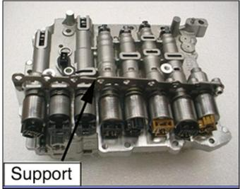
18. Refer to the DTC recorded in Step 1 and replace the related solenoid.
