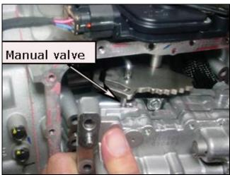
21. Install the valve body bolts and torque the bolts to specification in the order shown.
