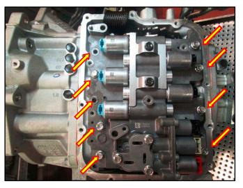
21. Reinstall the bolt that secures the detent spring and tighten the bolt to specification.
