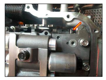
20. Install the valve body bolts and torque the bolts in order from the innermost bolts to the outermost bolts.
