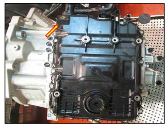
10. Remove 6 bolts to the harness and 1 bolt to the oil temperature sensor.
