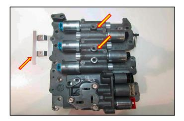
15. Refer to the DTC recorded in Step 1 and replace the related solenoid.
