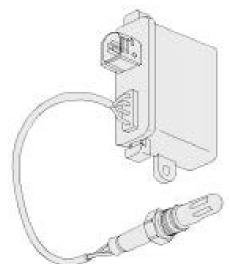
Installation torque of 50 Nm +/- 5
