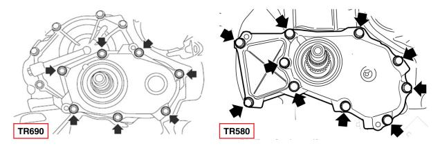
• Using a prying tool, **CAREFULLY** pry (GREEN arrows) the cover loose from the housing. Pry **ONLY** on the specific areas or "tabs" of the pump cover indicated by the BLUE arrows. When the cover starts to come loose, continue to pry ONLY on the tabs and not the machined sealing surface of the cover.
