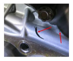
Take note of how the sealant on the removed cover forms an additional "seal" when it becomes displaced into the chamfer around the inside edge of the case's machined surface
