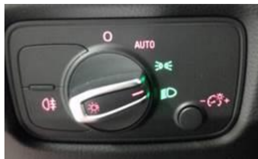
Figure 3. Switch in an intermediate position (2018 A4).
