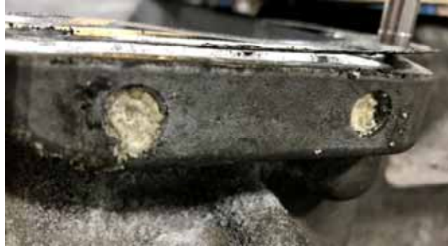
Clogged vent ports
