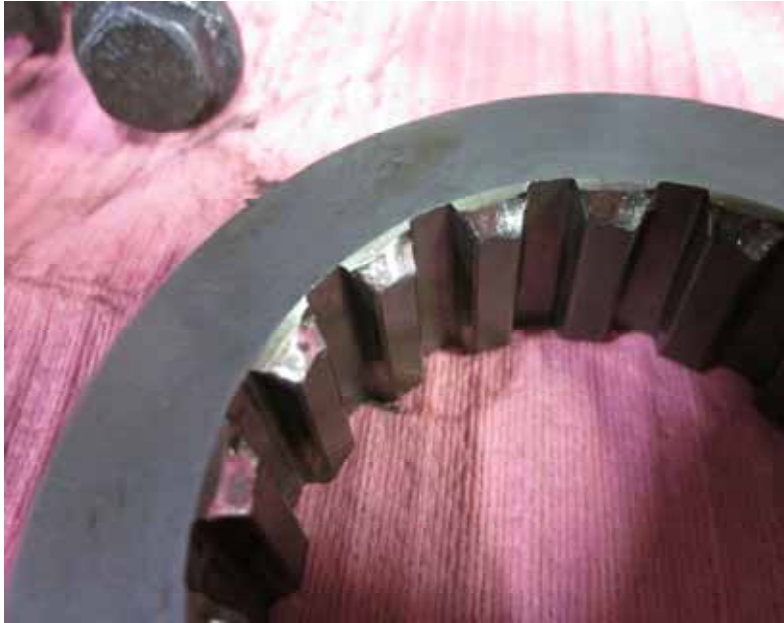
Spline and sliding clutch: Damaged components should be replaced
