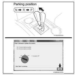
j) After "Flash Calibration Update Successful" is displayed, move the shift lever to Parking position and turn the IG off and click the "Next" button.
