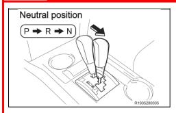
f) Turn the IG to the ON position (engine off).NOTE:DO NOT depress the brake pedal.
