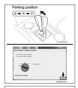
j) After "Flash Calibration Update Successful" is displayed, move the shift lever to Parking position and turn the IG off and click the "Next" button
