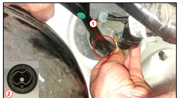
1 Cut at Grommet Indent Mark 2 Modified Grommet
