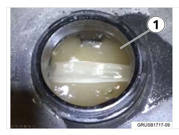
Coolant in the low temperature cooling circuit may also have an acrid smell and discoloration (1).
