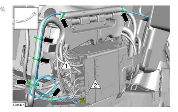
Route the new IMC rear link lead cable through the harness bracket and using suitable cable ties, secure it to the main wiring harness. Any excess cable must be looped '1' and secured to the main wiring harness. Connect the new IMC rear link lead cable to the IMC '2'.
