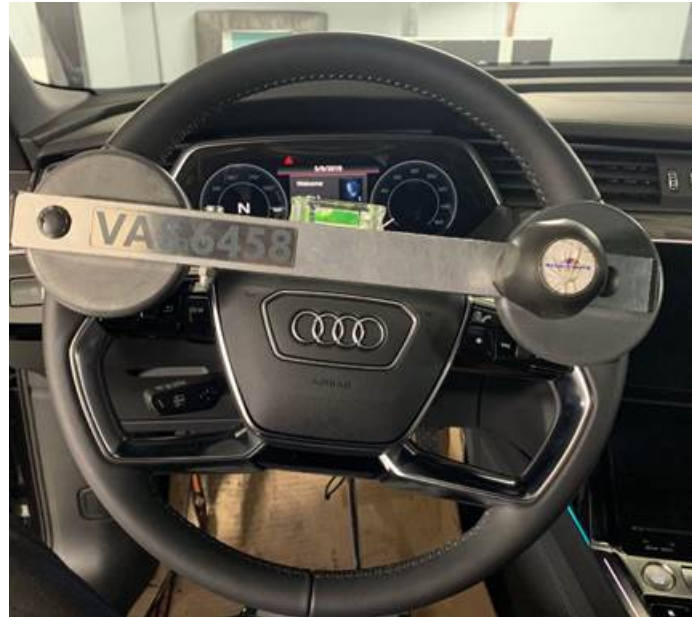
Figure 1. VAS 6458 installed with steering wheel off-center.
